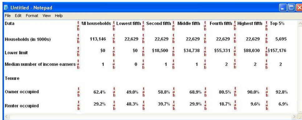
Figure 2 The way such a file really looks after being copied to a system's clipboard
